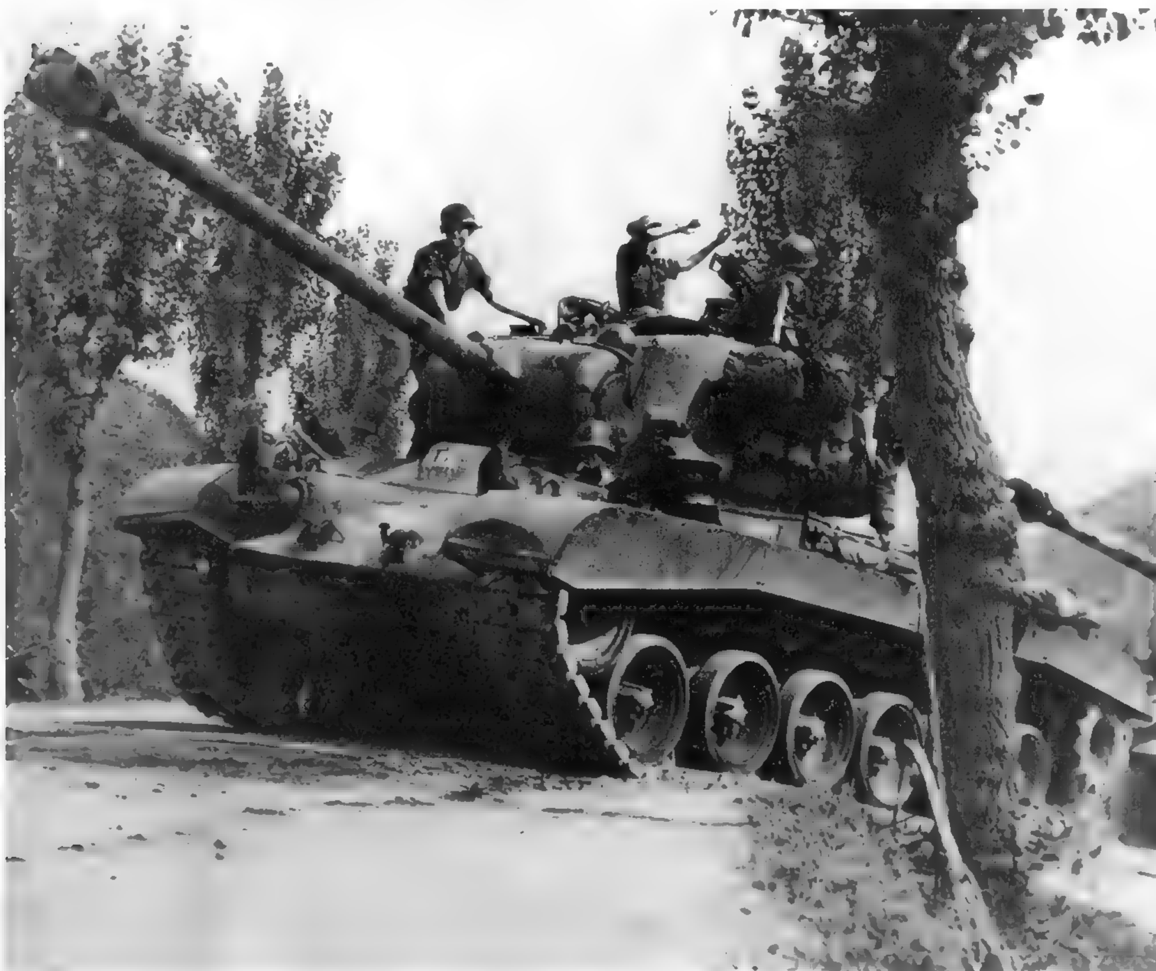
The bow machine gun can be seen on "Alice," an M26. The driver has his seat elevated so his head and shoulders are outside the hull, affording a much better view than the periscope. (U.S. Army photo)
